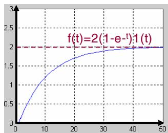
$$\begin{aligned} &= \lim_{T \rightarrow \infty} \frac{1}{2T} \int_0^T 4(1 - 2e^{-t} + e^{-2t}) dt = \lim_{T \rightarrow \infty} \frac{1}{2T} [4T + 8e^{-T} - 2e^{-2T}]_0^T \\ &= \lim_{T \rightarrow \infty} \frac{1}{2T} [4T + 8e^{-T} - 2e^{-2T} - 8 + 2] = 2 \end{aligned}$$
