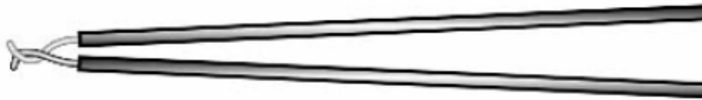
C. Insulated thermocouple twisted and welded
