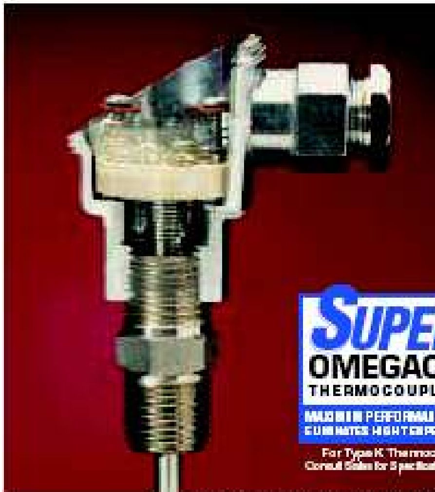
Cut-away of NB2 style to show detail of spring mechanism and terminal block.
