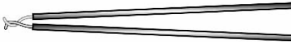
C. Insulated thermocouple twisted and welded
