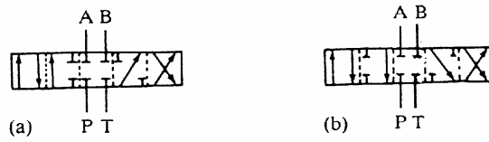
Figure 3.56 Spool transition states switching from center to end position. (a) Pressure port opening. (b) Tank port opening.
