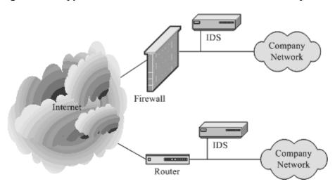
Figure 1-4. Typical locations for an intrusion detection system.
