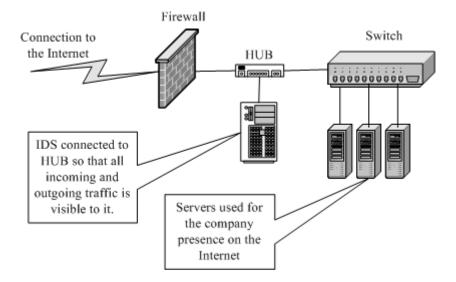
Note that when the IDS is connected as shown in <u>Figure 1-8</u>, data flowing among the company servers is not visible to the IDS. The IDS can see only that data which is coming from or going to the Internet. This is useful if you expect attacks from outside and the internal network is a trusted one.
