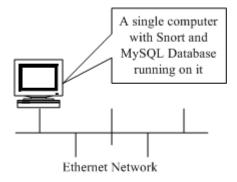
• You can also install the MySQL server on a different machine and configure Snort to log to that database, as shown in <u>Figure 5-2</u>.
