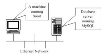
• You can have multiple Snort sensors to log to a centralized database server running MySQL server, as shown in Figure 5-3.
