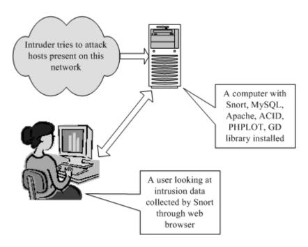
In the enterprise, usually people have multiple Snort sensors behind every router or firewall. In that case you can use a single centralized database to collect data from all of the sensors. You can run Apache web server on this centralized database server as shown in <u>Figure 1-3</u>.
