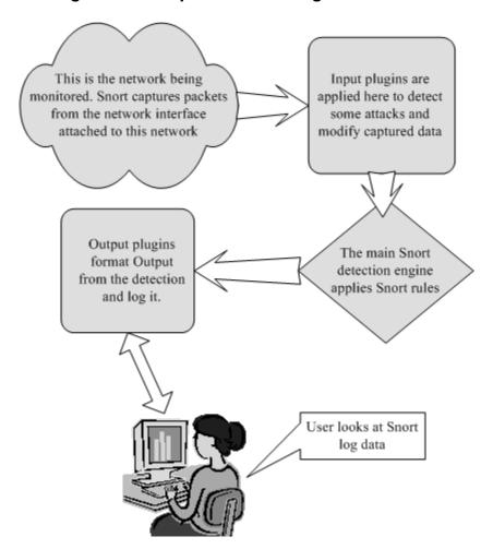
Figure 4-1. Simplified block diagram for Snort.
