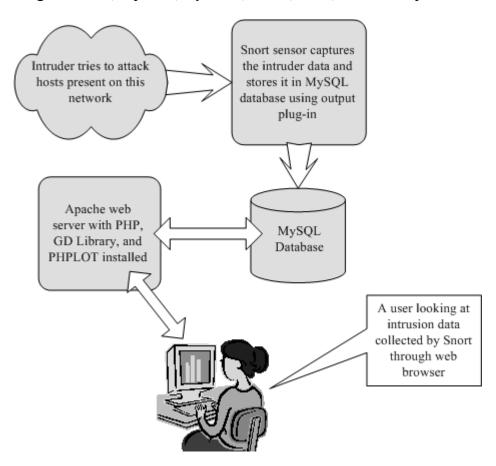
As you can see, data is captured and analyzed by Snort. Snort then stores this data in the MySQL database using the database output plug-in. Apache web server takes help from ACID, PHP, GD library and PHPLOT package to display this data in a browser window when a user connects to Apache. A user can then make different types of queries on the forms displayed in the web pages to analyze, archive, graph and delete data.
