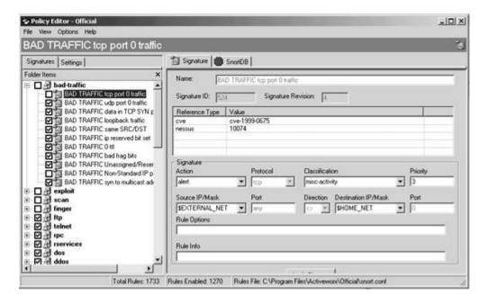
The pull-down menus in the right side of the window shown in <u>Figure 7-6</u> make it very easy to modify rules. For example, to modify protocol used in the rule, you can click the pull-down menu button and a list of supported protocols will appear.
