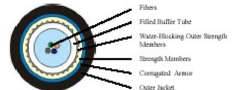
Central Loose Tube Armored Jacket
