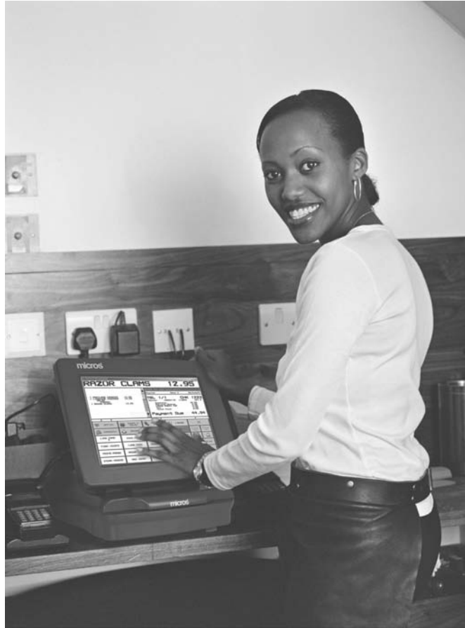
FIGURE 7-3 Touch Screen on Server Terminal: The server terminal may have a touch screen feature. The server merely touches the appropriate prompt on the screen to enter the order. Courtesy of MICROS® Systems, Inc.
