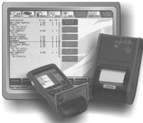
FIGURE 7-5 Handheld Order Terminal: Handheld order terminals can work with or replace the stationary server terminals in restaurants. Courtesy of Menusoft Systems, the developer of Digital Dining
