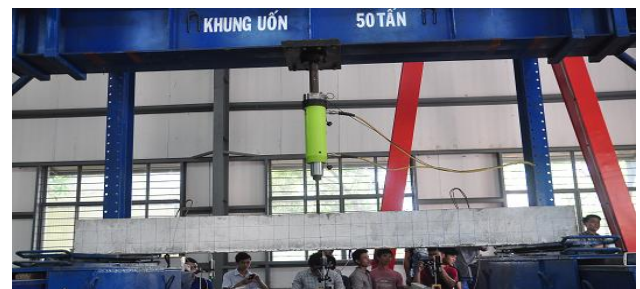
Fig.2. Bending test of beams.
