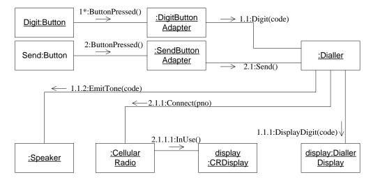
Figure 1: Collaboration diagram of Cellular Phone.
