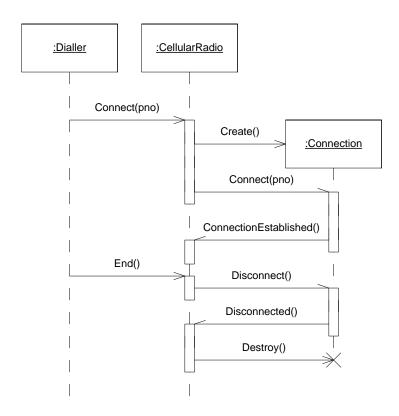
Figure 3: Connecting and Disconnecting
