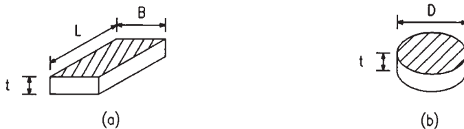
Fig. 28.2 Elastomeric bearing dimensions for (a) a rectangular block, (b) a circular block
