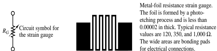
Figure 2.26 Metal-foil resistance strain gauge. The foil is formed by a photo-etching process and is less than 0.00002 in thick. Typical resistance values are 120, 350, and 1,000 \Omega . The wide areas are bonding pads for electrical connections.
