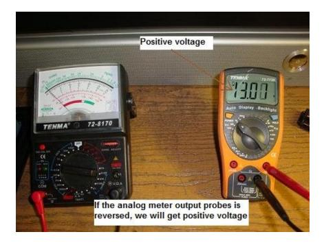
which is very good considering this meter only cost \$49.00 from MCM Electronics. This voltage is very good for turning on various components, but for some diodes this voltage can damage the PN junctions.
