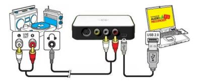
Connections from your audio player can be made via RCA (Composite) cables or with a Headphone-to-RCA (Composite) adapter cable.
