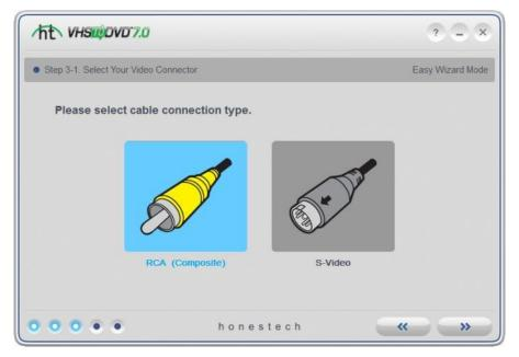
\*S-Video cables transmit a higher quality video signal than regular RCA (Composite) cables, but they do not carry an audio signal. RCA (Composite) audio cables are still required when making an S-Video connection.
