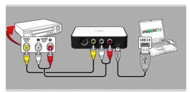
Connections from your video player can be made via RCA (Composite) cables (above), or with a combination of S-Video and RCA (Composite) audio cables (below).
