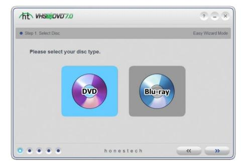
\*These are the types of discs the Wizard can record your video onto. The most common type used is DVD, however Blu-ray provides higher quality picture when played in a Blu-ray player. The Blu-ray option also requires a video signal from a HDV/DV (high definition video) camcorder.
