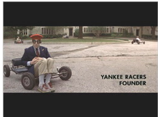
Anamorphic video as it appears on a Standard 4x3 TV. The DVD player performs a mathematical downconversion on the video signal, in effect combining every 4 lines of vertical resolution into 3 until the correct aspect ratio is achieved. Electronically-generated black bars are added to the existing ones (to fill in the remaining screen area), completing the image. Visually, it's nearly indistinguishable from a non-anamorphic (letterboxed) DVD image.
