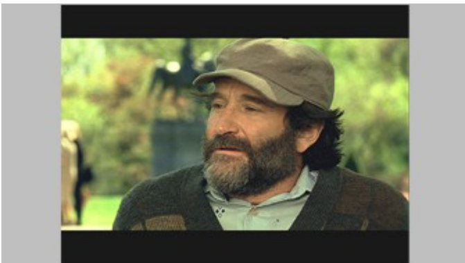
Non-anamorphic video as it appears on a Digital 16x9 TV. The gray bars are generated by the TV to fill in the unused portions of the screen. Using the TV's "zoom" mode, you can magnify the image to fill the screen electronically, but at the cost of degrading the image quality significantly.
