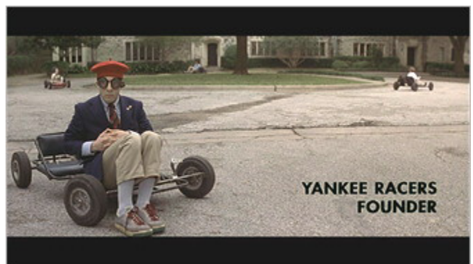
Anamorphic video as it appears on a Digital 16x9 TV. The "squished" image recorded on the disc (seen at top) is sent directly to the TV, which stretches the video signal horizontally until the correct aspect ratio is achieved. As you can see, the image fills the frame, while retaining nearly its full vertical resolution. Since the 2.35:1 aspect ratio is wider, thin black bars are still necessary to maintain the proper composition (they're in the video signal). The picture quality is stunning.
