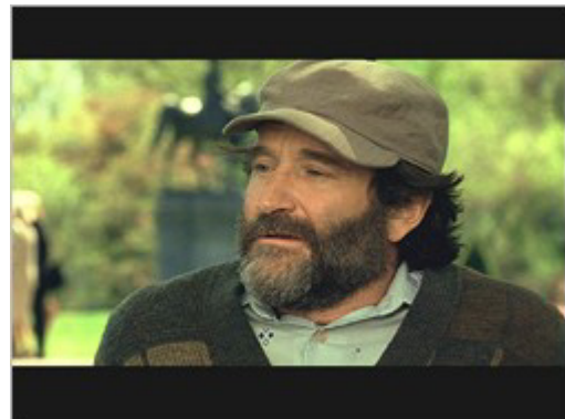
Anamorphic video as it appears on a Standard 4x3 TV. The DVD player performs a mathematical downconversion on the video signal, in effect combining every 4 lines of vertical resolution into 3 until the correct aspect ratio is achieved. The black bars at the top and bottom of the image are generated electronically, completing the image. Visually, it's nearly indistinguishable from a non-anamorphic (letterboxed) DVD image.
