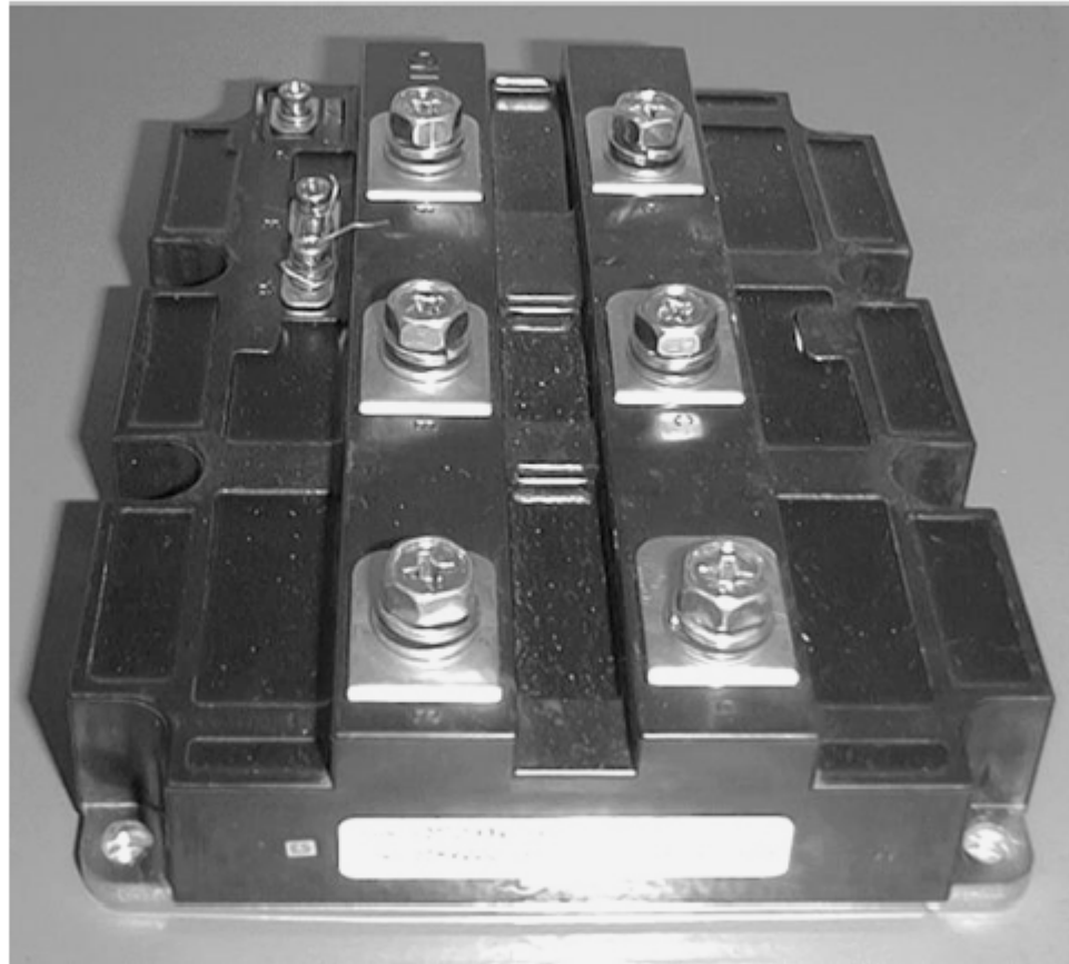
FIGURE 1.89 Photograph of a 1200-A, 3300-V IGBT module in which 24 1-cm 2 IGBT dies are paralleled together by wire bonds.
