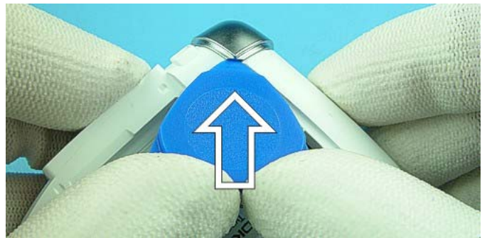
The Corner Piece fits very tight, so it needs some extra force to separate it from B-Cover with SRT-6.
