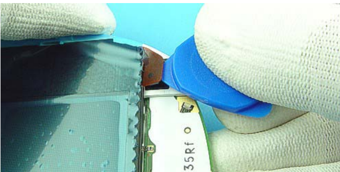
Carefully open LCD Connector with SRT-6. Do not damage the sensitive flex foil.
