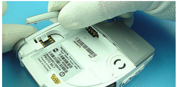
Pull up D-Cover, which is attached to B-Cover with adhesive tape.
