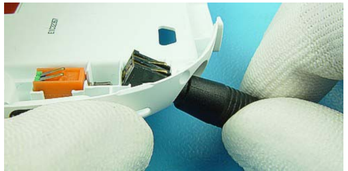
Take a charger plug to remove DC Jack.
