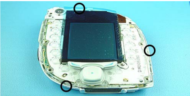
Unlock the three clips from UI Assy as shown in the next picture.
