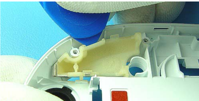
Lever out WCDMA Antenna from B-Cover.
