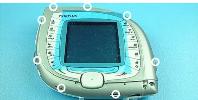
A-Cover is fixed with several plastic clips. Start with the clip near system connector.
