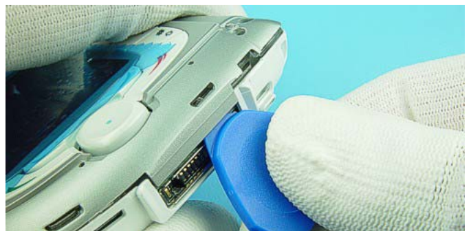
Loosen the clips anti-clockwise by using the SRT-6 as a lever. Do not twist SRT-6 because this could cause damages to the covers.
