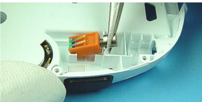
Do not damage the spring contacts when removing Vibra Motor.
