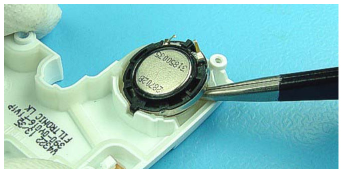
Finally remove HF Speaker with tweezers.
