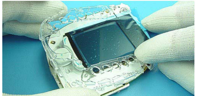
After opening the side clips the Lightguide can be taken away.
