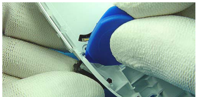
Unlock the side snaps to remove IR Window.
