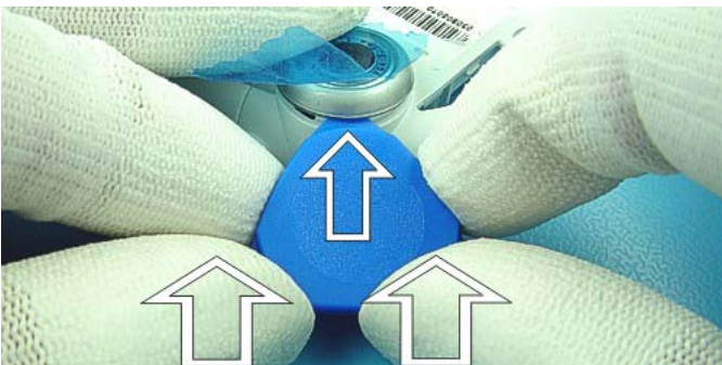
Detach Camera Window by placing SRT-6 as shown and pressing upwards forcefully.
