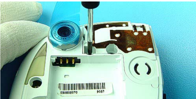
Unscrew Antenna screw. Use a new Torx Plus® screw and a torque of 24 Ncm for assembling the old B-Cover and use 26 Ncm when using a new B-Cover.
