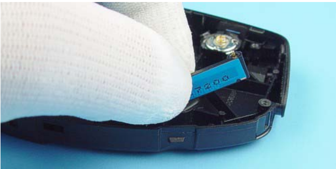
Now, the Antenna can be removed easily.
