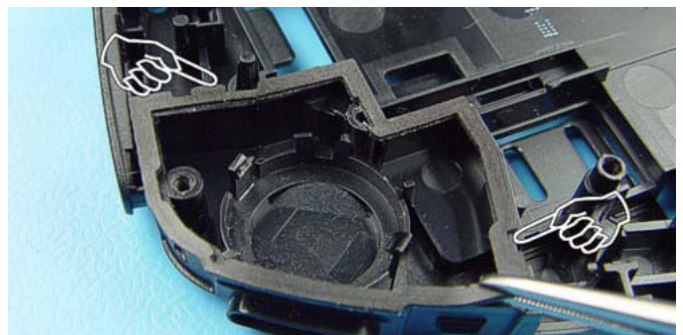
Replace the Silicone Gasket with a new one. Note the right position.
