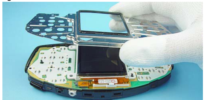
Now, the UI-Shield can be taken away. Protect the LCD Module with a film to avoid dust und scratches.
