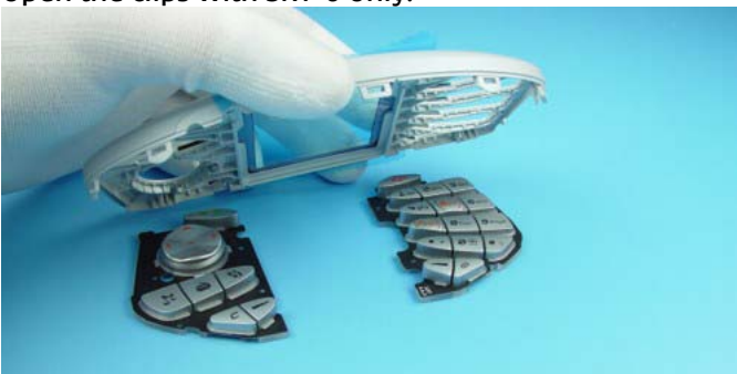
Both Keymats drop out when turning A-Cover.
