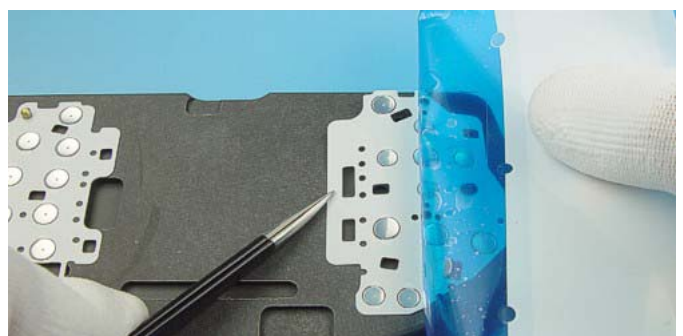
Use the same procedure also for the Dome Sheet Left.
