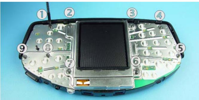
Unscrew the nine Torx Plus® size 6 screws using the order shown. For assembly, the reverse order and a Torx Plus® driver with a torque of 26Ncm have to be used.
