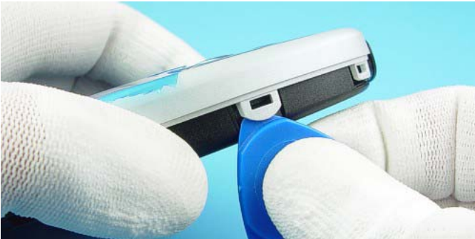
A-Cover is attached with two main clips to the Chassis. Open the clips with SRT-6 only.
