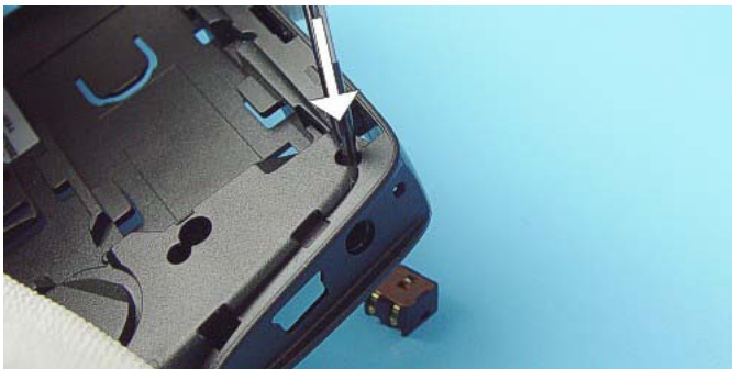
Remove Microphone by pushing a Torx driver through this opening.
