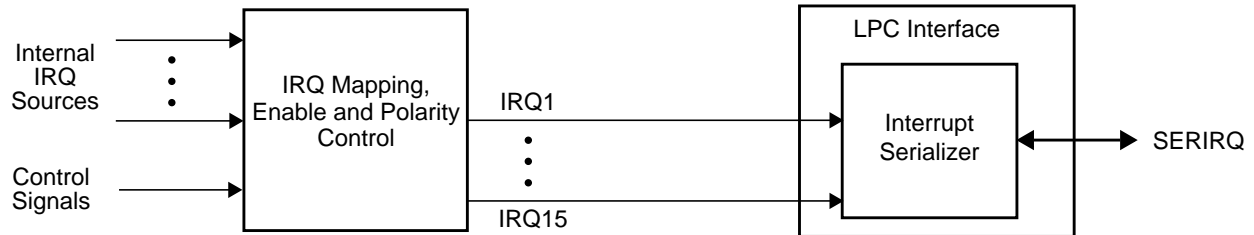
Figure 111. Interrupt Serialization Mechanism
