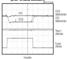
ICTL = 3.30V CHARGING CURRENT = 2.0A V<sub>BATT</sub> = 16V LOAD STEP = 0 TO 3A ISOURCE LIMIT = 5A
