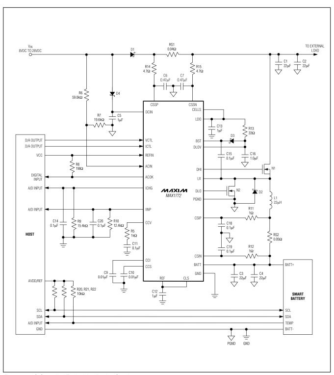
Figure 1a. µC-Controlled Typical Application Circuit
