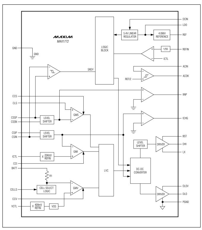
Figure 2. Functional Diagram
