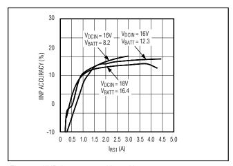
Figure 3. IINP Accuracy vs. VDCIN/VBATT
