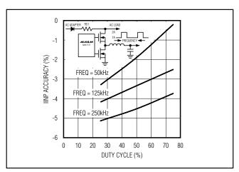
Figure 4. IINP Accuracy vs. AC Load Duty Cycle
