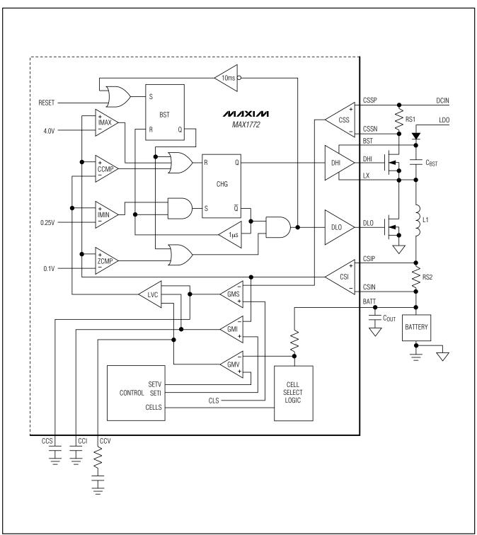
Figure 5. DC-to-DC Converter Functional Diagram
