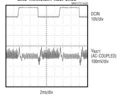
V<sub>BATT</sub> = 16V DCIN = 18.5V TO 27.5V  $I_{LOAD} = 150 \text{mA}$
