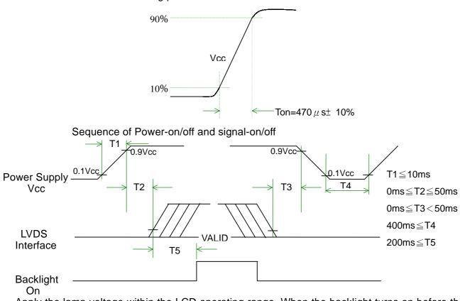
Apply the lamp voltage within the LCD operating range. When the backlight turns on before the LCD operation or the LCD turns off before the backlight turns off, the display may momentarily become abnormal.
