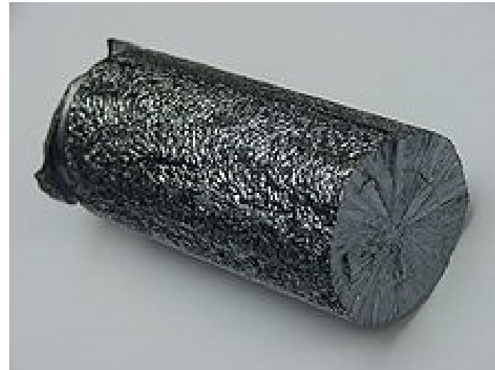
A polycrystalline silicon rod made by the Siemens process
