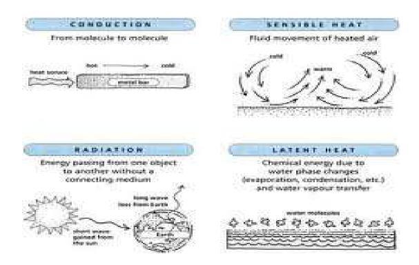
Heat flows from a substance of higher temperature to bodies of lower temperature in the same manner that water flows down a hill, and like water, it can be raised again to a higher level so that it may repeat its cycle.
