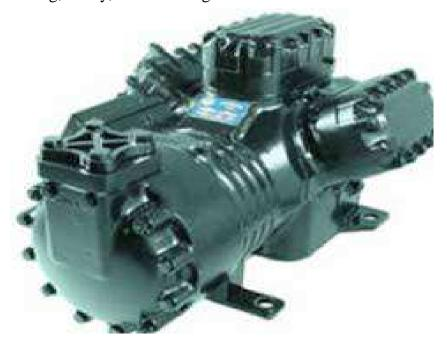
**External Drive Compressor**. — An external drive or open-type compressor is bolted together. Its crankshaft extends through the crankcase and is driven by a flywheel (pulley) and belt, or it can be driven directly by an electric motor.
