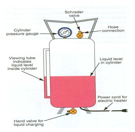
To transfer refrigerants, connect a flexible charging line on a 1/4-inch copper tube several feet long with a circular loop about 8 to 10 inches in
