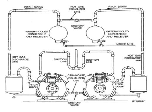
Water-cooled condensers require a free area equal to the length of the condenser at one end to provide room for cleaning tubes, installing new tubes, or removal of the condenser tube assembly. Space is needed for servicing
