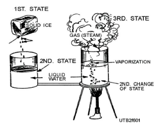
When heat is added to a substance, the rate of molecular motion increases, causing the substance to change from a solid to a liquid, and then to a gas (vapor). For example, in a cube of ice, molecular motion is slow, but as heat is added, molecular activity increases, changing the solid "ice" to a liquid "water" (Fig. 6-1).
