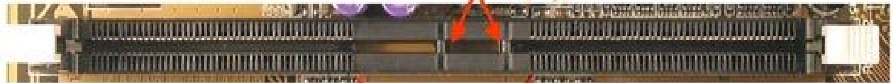
16-bit RIMM Connector (184 pins)
