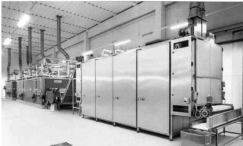
Fig. 9. Pre-dryer and dryer modular design (courtesy of Sandvik Process Systems, 1996).
