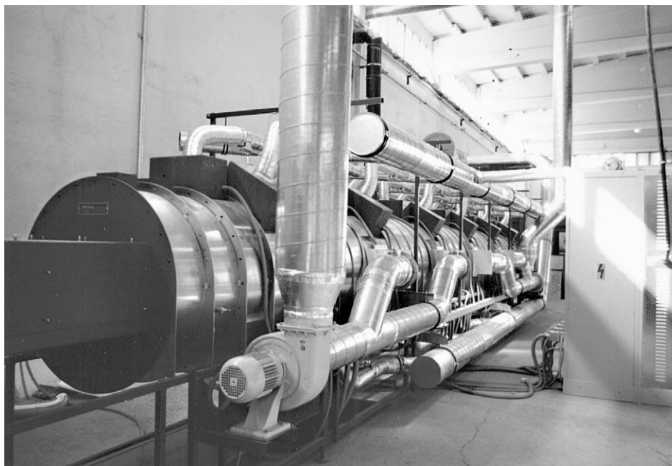
Fig. 27. Continuous microwave belt furnace 15 m and 60 kW (courtesy of Linn High Therm GmbH, 2000).
