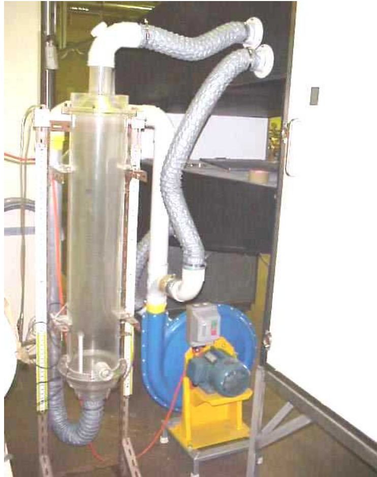
Figure 1 Fluidised bed experimental setup
