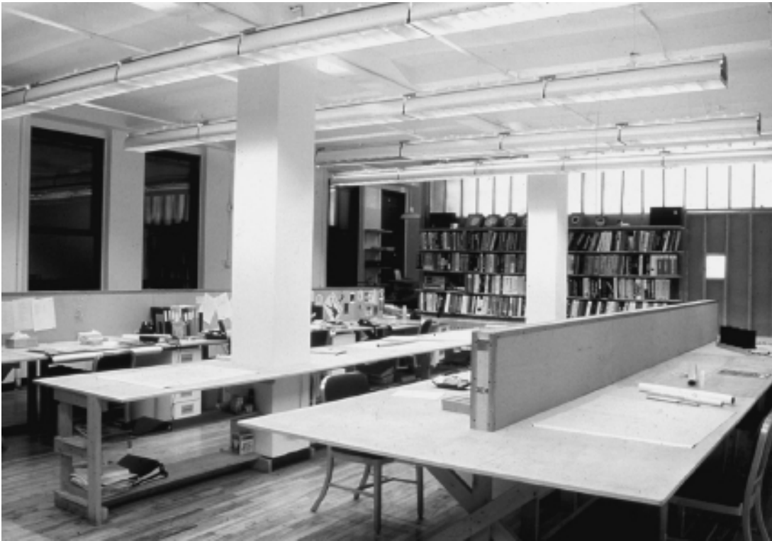
Figure 13.1 Low-brightness louvers minimize clutter on the ceiling and establish the primary focus in the activity portions of the visual field.
