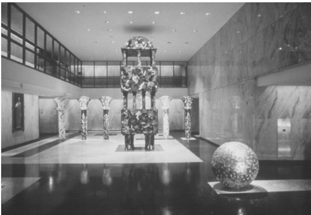
Figure 13.3 Matching luminaire apertures of the same dimension and finish.
