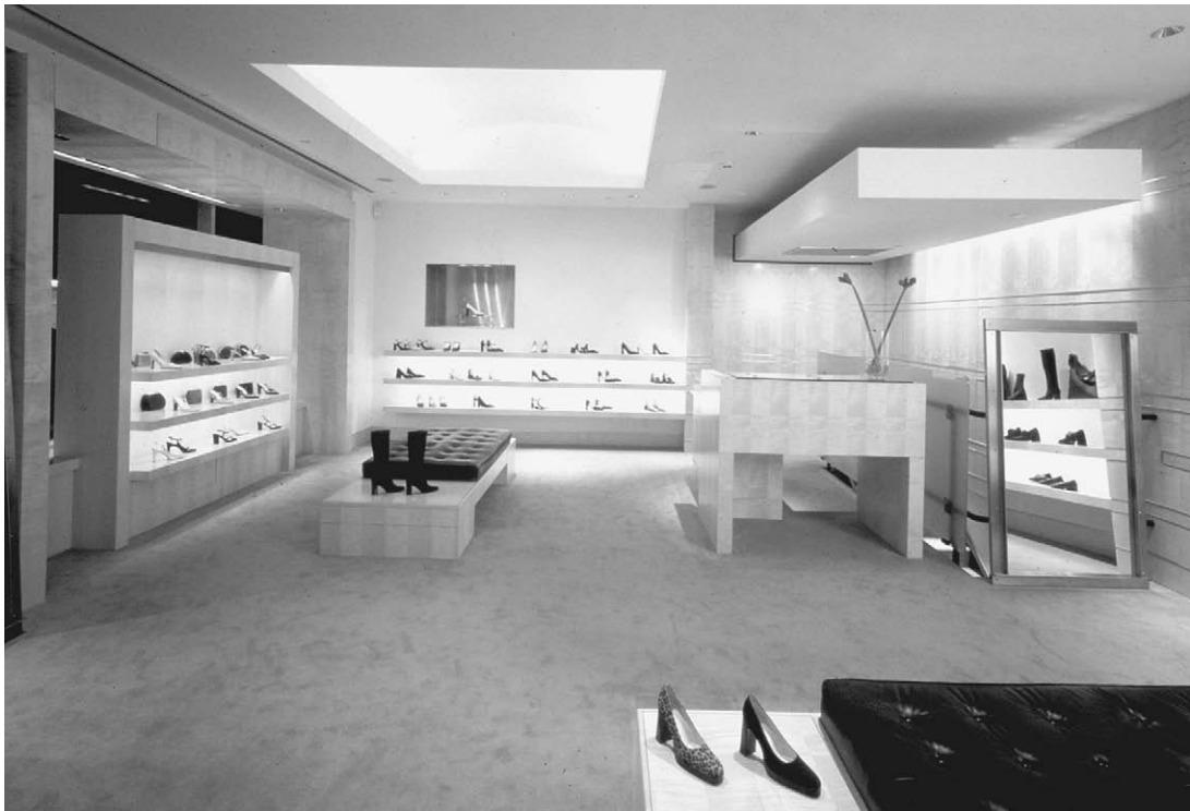
Figure 13.29 When lighted walls are distant from each other in a low-ceilinged space, downlighting added to the center provides balance of brightness.
