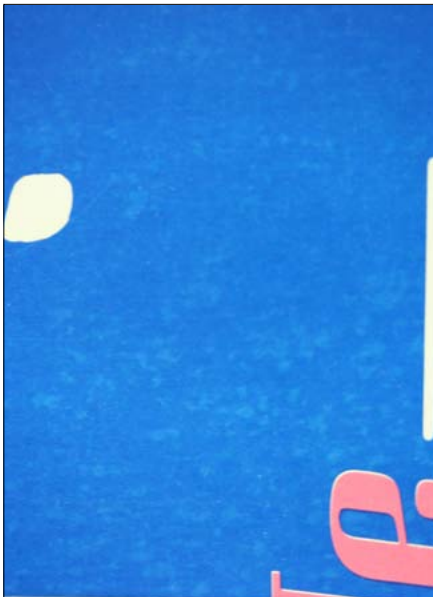
Fig. 32: Close focus image of mottling from a four-colour sheet-fed offset press.
