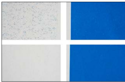
Fig. 26: Comparison of two different inks in a stack test. The upper sample clearly shows set-off marks due to its slower setting speed, compared to the test sample below.
