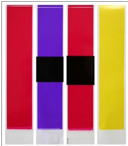
Fig. 14: Proof stripes: Outer pair for measurements of chromaticity coordinates, inner pair with black bar for determining the transparency.
