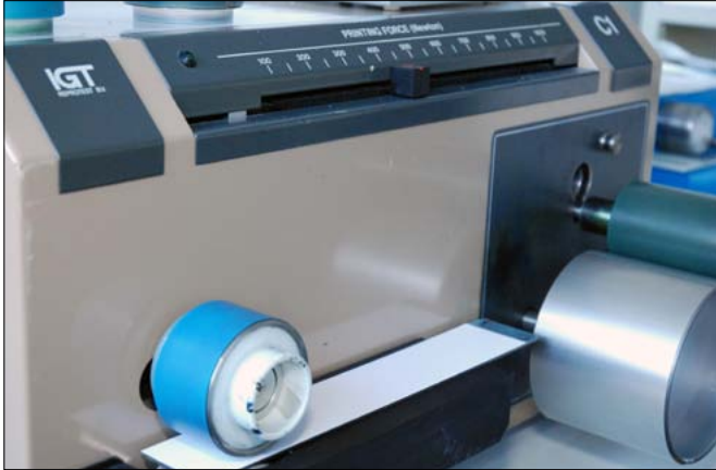
Fig. 13: Multi-purpose printability tester for proof printing
