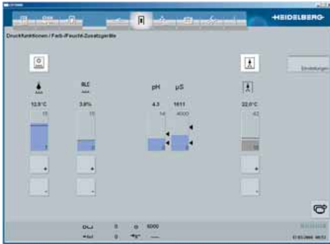
Temperature control made easy: thanks to CANopen, the temperature of the dampening solution can be set right at the Prinect CP2000 Center.
