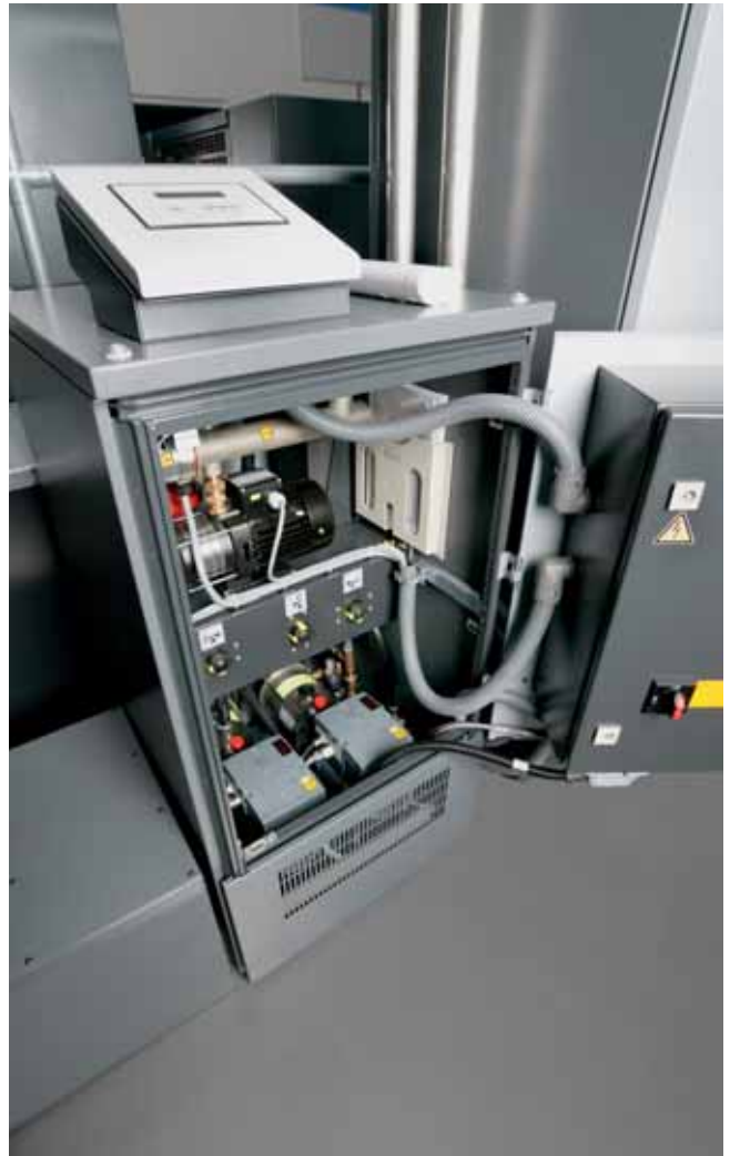
The CoatingStar as the universal coating supply unit is designed to accept all well-known types of coatings: two-roller system, chamber doctor blade or Flexokit.
