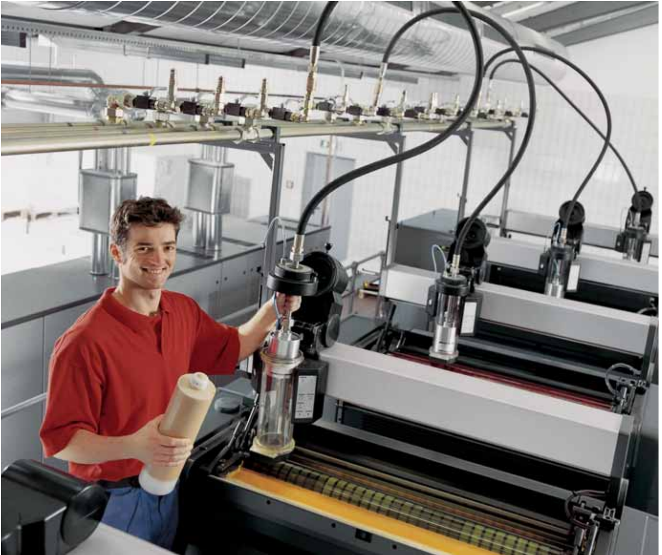
Flexible ink supply: InkLine takes either cartridges or a valve insert for connecting to a central ink supply source.
