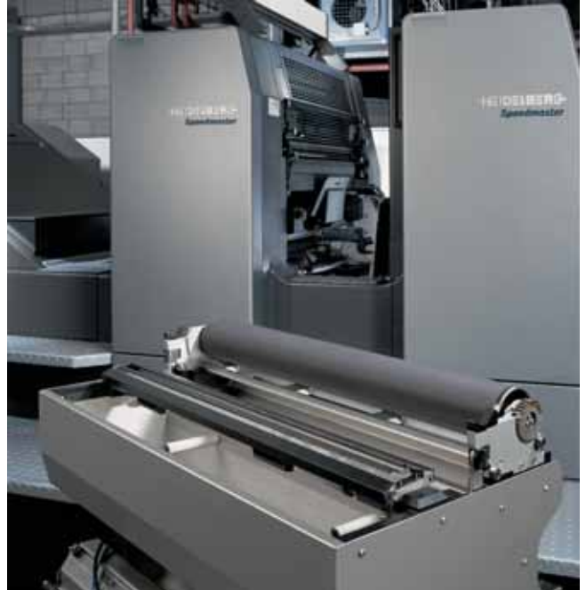
Additional flexibility for commercial printers: The MCS allows to conveniently apply water-based varnish in an offset printing unit.
