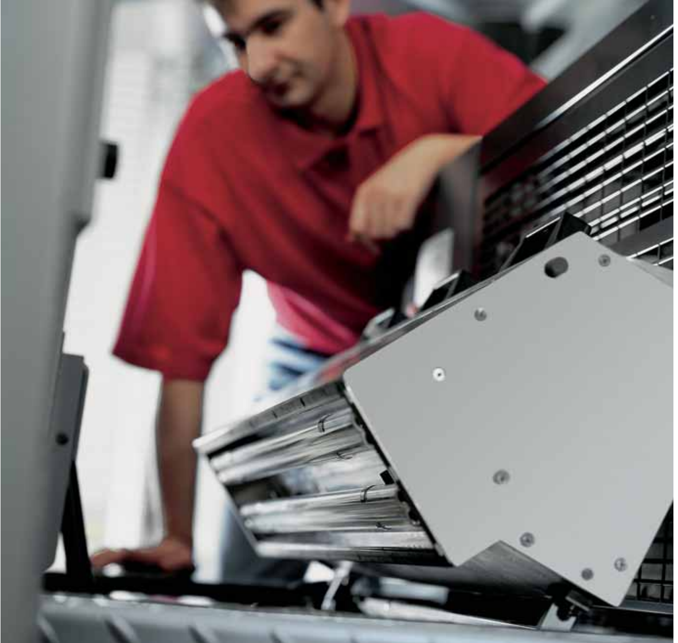
The DryStar UV interdeck dryer on the CD 74 can be pivoted up out of the way for easy cleaning of the transfer cylinder.
