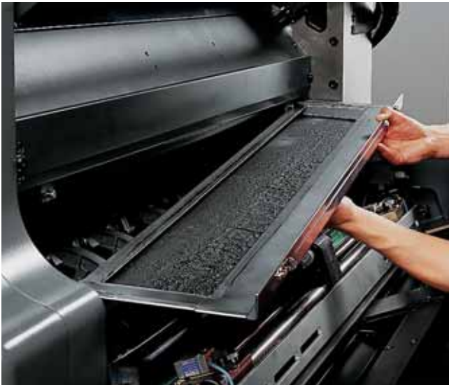
Without WashStar: manual cleaning of the catch pans required.
