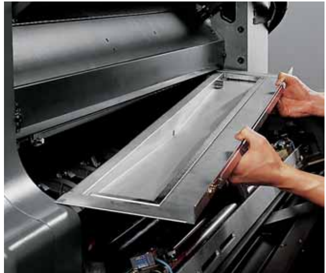
With WashStar: automatic rinsing keeps the catch pans clean.
