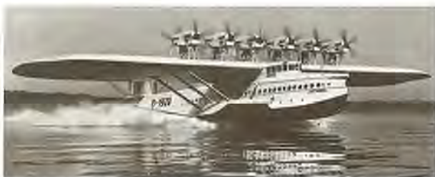
The Dornier Do X was a huge 12-engined flying boat which was much publicized but never a commercial success.
