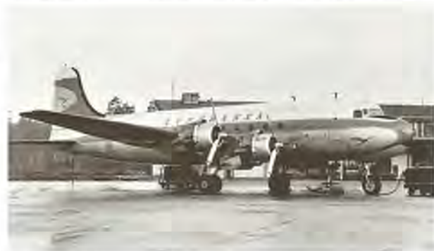
A Douglas C-54 cargo aircraft, used by Lufthansa for its first all-cargo flights.
