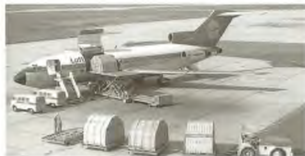
The Boeing 727-30QC , the "quick-change" mixed passenger-cargo version.
