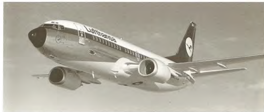
The Boeing 737-300 . The engine intakes are flattened for ground clearance.
