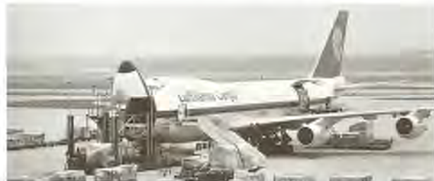
Lufthansa's Boeing 747F is loaded through both the nose and fuselage cargo doors.
