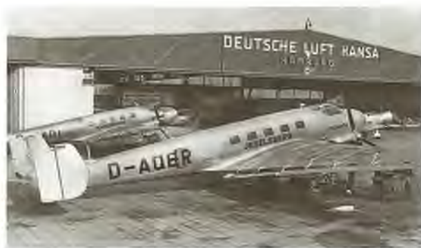
The Junkers-Ju 86 , built as both a commercial and a military aircraft.
