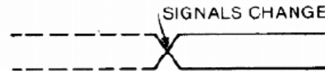
LOGIC STATES OF BUS SIGNALS ARE UNIMPORTANT PRIOR TO TIME THAT THEY CHANGE
