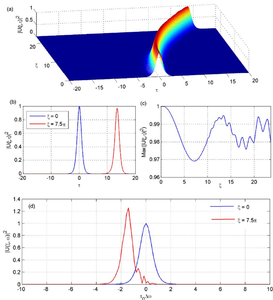
**Figure 2.** Effects of Raman scattering on fundamental soliton.
