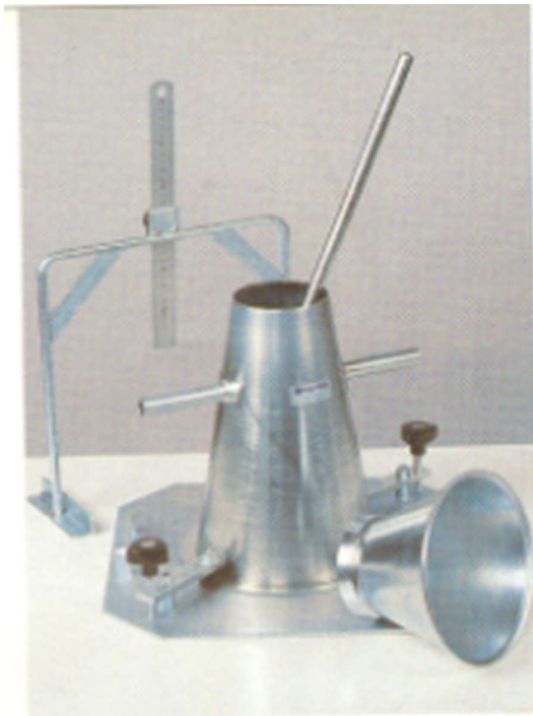
Slump cone with portal
