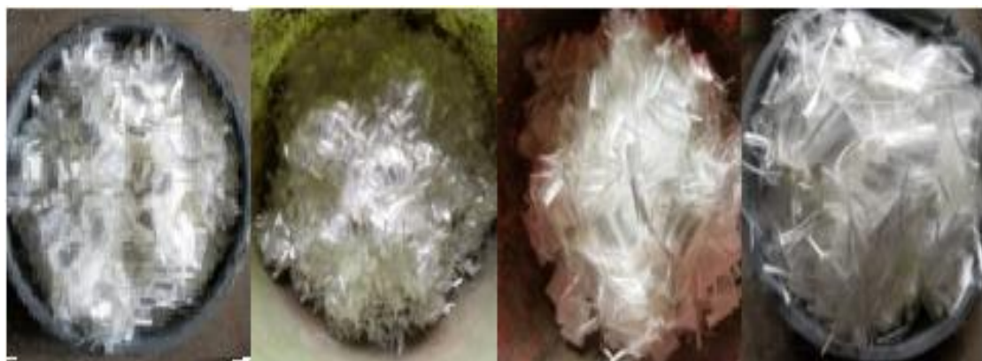
Sợi PP 10mm Sợi PP 20mm Sợi PP 35mm Sợi PP 50mm
