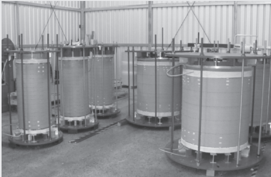
Figure 2 Good quality coils are essential to ensure the longevity of your transformer
