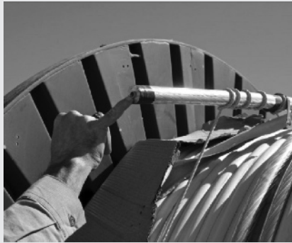
Figure 3 High-capacity low-sag conductor.
